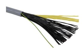
Southwire flexible control cable, unshielded, 41 conductors (includes ground), 16 AWG, bare copper, PVC/Nylon conductor insulation material, black with white numbers and green/yellow ground, TPE jacket, gray, cut to length.
