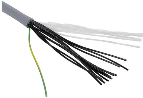
Southwire flexible control cable, unshielded, 12 conductors (includes ground), 16 AWG, bare copper, PVC/Nylon conductor insulation material, black with white numbers and green/yellow ground, TPE jacket, gray, cut to length.
