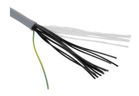
Southwire flexible control cable, unshielded, 12 conductors (includes ground), 16 AWG, bare copper, PVC/Nylon conductor insulation material, black with white numbers and green/yellow ground, TPE jacket, gray, cut to length.
