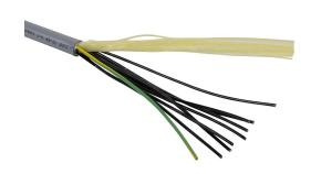
Southwire flexible control cable, unshielded, 9 conductors (includes ground), 16 AWG, bare copper, PVC/Nylon conductor insulation material, black with white numbers and green/yellow ground, TPE jacket, gray, cut to length.
