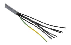
Southwire flexible control cable, unshielded, 7 conductors (includes ground), 16 AWG, bare copper, PVC/Nylon conductor insulation material, black with white numbers and green/yellow ground, TPE jacket, gray, cut to length.
