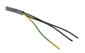
Southwire flexible control cable, unshielded, 3 conductors (includes ground), 16 AWG, bare copper, PVC/Nylon conductor insulation material, black with white numbers and green/yellow ground, TPE jacket, gray, cut to length.
