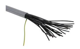
Southwire flexible control cable, unshielded, 25 conductors (includes ground), 18 AWG, bare copper, PVC/Nylon conductor insulation material, black with white numbers and green/yellow ground, TPE jacket, gray, cut to length.
