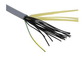
Southwire flexible control cable, unshielded, 18 conductors (includes ground), 18 AWG, bare copper, PVC/Nylon conductor insulation material, black with white numbers and green/yellow ground, TPE jacket, gray, cut to length.
