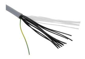
Southwire flexible control cable, unshielded, 12 conductors (includes ground), 18 AWG, bare copper, PVC/Nylon conductor insulation material, black with white numbers and green/yellow ground, TPE jacket, gray, cut to length.
