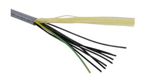
Southwire flexible control cable, unshielded, 9 conductors (includes ground), 18 AWG, bare copper, PVC/Nylon conductor insulation material, black with white numbers and green/yellow ground, TPE jacket, gray, cut to length.
