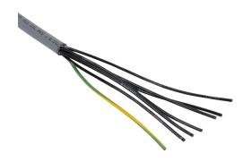
Southwire flexible control cable, unshielded, 7 conductors (includes ground), 18 AWG, bare copper, PVC/Nylon conductor insulation material, black with white numbers and green/yellow ground, TPE jacket, gray, cut to length.
