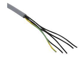
Southwire flexible control cable, unshielded, 5 conductors (includes ground), 18 AWG, bare copper, PVC/Nylon conductor insulation material, black with white numbers and green/yellow ground, TPE jacket, gray, cut to length.
