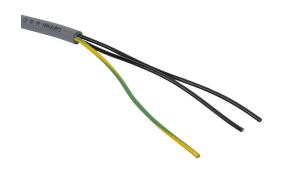
Southwire flexible control cable, unshielded, 3 conductors (includes ground), 18 AWG, bare copper, PVC/Nylon conductor insulation material, black with white numbers and green/yellow ground, TPE jacket, gray, cut to length.
