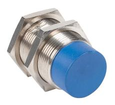
Micro Detectors inductive proximity sensor, tubular, 30mm diameter x 60mm body, nickel-plated brass housing, N.C. (VAC) or N.O./N.C. (VDC) output, 18mm sensing distance, non-flush, 25 Hz (AC)/190 Hz (DC) switching frequency, IP67, 1/2in - 20UNF thread.
