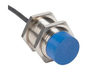
Micro Detectors inductive proximity sensor, tubular, 30mm diameter x 55mm body, nickel-plated brass housing, N.C. (VAC) or N.O./N.C. (VDC) output, 18mm sensing distance, non-flush, 25 Hz (AC)/190 Hz (DC) switching frequency, IP67, pigtail.
