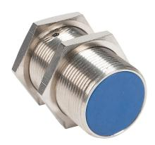
Micro Detectors inductive proximity sensor, tubular, 30mm diameter x 60mm body, nickel-plated brass housing, N.C. (VAC) or N.O./N.C. (VDC) output, 12mm sensing distance, flush, 25 Hz (AC)/250 Hz (DC) switching frequency, IP67, 1/2in - 20UNF thread.
