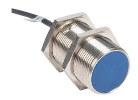
Micro Detectors inductive proximity sensor, tubular, 30mm diameter x 55mm body, nickel-plated brass housing, N.C. (VAC) or N.O./N.C. (VDC) output, 12mm sensing distance, flush, 25 Hz (AC)/250 Hz (DC) switching frequency, IP67, pigtail.
