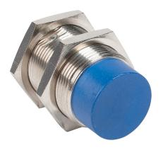
Micro Detectors inductive proximity sensor, tubular, 30mm diameter x 60mm body, nickel-plated brass housing, N.O. (VAC) or N.O./N.C. (VDC) output, 18mm sensing distance, non-flush, 25 Hz (AC)/190 Hz (DC) switching frequency, IP67, 1/2in - 20UNF thread.
