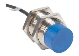
Micro Detectors inductive proximity sensor, tubular, 30mm diameter x 55mm body, nickel-plated brass housing, N.O. (VAC) or N.O./N.C. (VDC) output, 18mm sensing distance, non-flush, 25 Hz (AC)/190 Hz (DC) switching frequency, IP67, pigtail.
