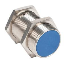
Micro Detectors inductive proximity sensor, tubular, 30mm diameter x 60mm body, nickel-plated brass housing, N.O. (VAC) or N.O./N.C. (VDC) output, 12mm sensing distance, flush, 25 Hz (AC)/250 Hz (DC) switching frequency, IP67, 1/2in - 20UNF thread.
