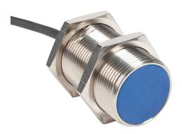
Micro Detectors inductive proximity sensor, tubular, 30mm diameter x 55mm body, nickel-plated brass housing, N.O. (VAC) or N.O./N.C. (VDC) output, 12mm sensing distance, flush, 25 Hz (AC)/250 Hz (DC) switching frequency, IP67, pigtail.
