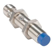
Micro Detectors inductive proximity sensor, tubular, 12mm diameter x 65mm body, nickel-plated brass housing, N.C. (VAC) or N.O./N.C. (VDC) output, 6mm sensing distance, non-flush, 25 Hz (AC)/500 Hz (DC) switching frequency, IP67, 1/2in - 20UNF thread.
