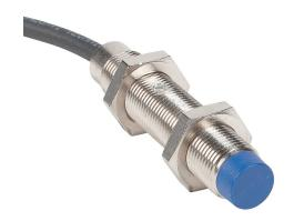
Micro Detectors inductive proximity sensor, tubular, 12mm diameter x 60mm body, nickel-plated brass housing, N.C. (VAC) or N.O./N.C. (VDC) output, 6mm sensing distance, non-flush, 25 Hz (AC)/500 Hz (DC) switching frequency, IP67, pigtail.
