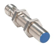
Micro Detectors inductive proximity sensor, tubular, 12mm diameter x 65mm body, nickel-plated brass housing, N.C. (VAC) or N.O./N.C. (VDC) output, 4mm sensing distance, flush, 25 Hz (AC)/750 Hz (DC) switching frequency, IP67, 1/2in - 20UNF thread.
