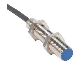
Micro Detectors inductive proximity sensor, tubular, 12mm diameter x 60mm body, nickel-plated brass housing, N.C. (VAC) or N.O./N.C. (VDC) output, 4mm sensing distance, flush, 25 Hz (AC)/750 Hz (DC) switching frequency, IP67, pigtail.
