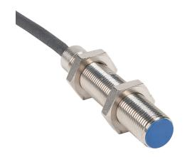
Micro Detectors inductive proximity sensor, tubular, 12mm diameter x 60mm body, nickel-plated brass housing, N.C. (VAC) or N.O./N.C. (VDC) output, 4mm sensing distance, flush, 25 Hz (AC)/750 Hz (DC) switching frequency, IP67, pigtail.
