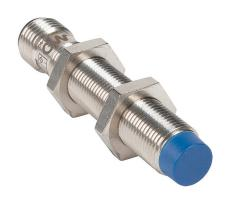
Micro Detectors inductive proximity sensor, tubular, 12mm diameter x 65mm body, nickel-plated brass housing, N.O. (VAC) or N.O./N.C. (VDC) output, 6mm sensing distance, non-flush, 25 Hz (AC)/500 Hz (DC) switching frequency, IP67, 1/2in - 20UNF thread.
