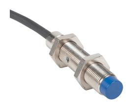
Micro Detectors inductive proximity sensor, tubular, 12mm diameter x 60mm body, nickel-plated brass housing, N.O. (VAC) or N.O./N.C. (VDC) output, 6mm sensing distance, non-flush, 25 Hz (AC)/500 Hz (DC) switching frequency, IP67, pigtail.
