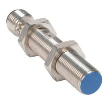
Micro Detectors inductive proximity sensor, tubular, 12mm diameter x 65mm body, nickel-plated brass housing, N.O. (VAC) or N.O./N.C. (VDC) output, 4mm sensing distance, flush, 25 Hz (AC)/750 Hz (DC) switching frequency, IP67, 1/2in - 20UNF thread.
