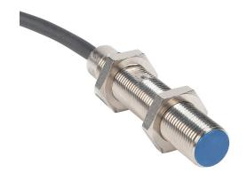
Micro Detectors inductive proximity sensor, tubular, 12mm diameter x 60mm body, nickel-plated brass housing, N.O. (VAC) or N.O./N.C. (VDC) output, 4mm sensing distance, flush, 25 Hz (AC)/750 Hz (DC) switching frequency, IP67, pigtail.
