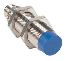
Micro Detectors inductive proximity sensor, tubular, 18mm diameter x 64.5mm body, nickel-plated brass housing, N.C. (VAC) or N.O./N.C. (VDC) output, 10mm sensing distance, non-flush, 25 Hz (AC)/550 Hz (DC) switching frequency, IP67, 1/2in - 20UNF thread.
