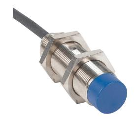
Micro Detectors inductive proximity sensor, tubular, 18mm diameter x 60mm body, nickel-plated brass housing, N.C. (VAC) or N.O./N.C. (VDC) output, 10mm sensing distance, non-flush, 25 Hz (AC)/550 Hz (DC) switching frequency, IP67, pigtail.
