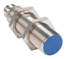
Micro Detectors inductive proximity sensor, tubular, 18mm diameter x 64.5mm body, nickel-plated brass housing, N.C. (VAC) or N.O./N.C. (VDC) output, 6mm sensing distance, flush, 25 Hz (AC)/600 Hz (DC) switching frequency, IP67, 1/2in - 20UNF thread.
