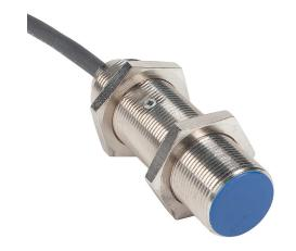
Micro Detectors inductive proximity sensor, tubular, 18mm diameter x 60mm body, nickel-plated brass housing, N.C. (VAC) or N.O./N.C. (VDC) output, 6mm sensing distance, flush, 25 Hz (AC)/600 Hz (DC) switching frequency, IP67, pigtail.
