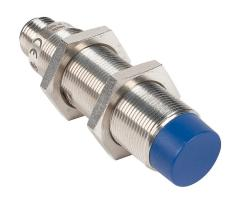
Micro Detectors inductive proximity sensor, tubular, 18mm diameter x 64.5mm body, nickel-plated brass housing, N.O. (VAC) or N.O./N.C. (VDC) output, 10mm sensing distance, non-flush, 25 Hz (AC)/550 Hz (DC) switching frequency, IP67, 1/2in - 20UNF thread.
