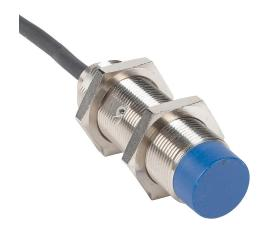
Micro Detectors inductive proximity sensor, tubular, 18mm diameter x 60mm body, nickel-plated brass housing, N.O. (VAC) or N.O./N.C. (VDC) output, 10mm sensing distance, non-flush, 25 Hz (AC)/550 Hz (DC) switching frequency, IP67, pigtail.
