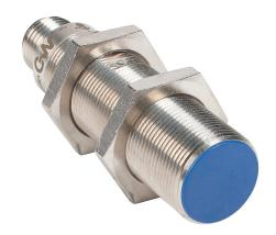
Micro Detectors inductive proximity sensor, tubular, 18mm diameter x 64.5mm body, nickel-plated brass housing, N.O. (VAC) or N.O./N.C. (VDC) output, 6mm sensing distance, flush, 25 Hz (AC)/600 Hz (DC) switching frequency, IP67, 1/2in - 20UNF thread.
