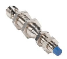
Micro Detectors inductive proximity sensor, tubular, 8mm diameter x 82mm body, nickel-plated brass housing, N.C. (VAC) or N.O./N.C. (VDC) output, 4mm sensing distance, non-flush, 25 Hz (AC)/750 Hz (DC) switching frequency, IP67, 1/2in - 20UNF thread.
