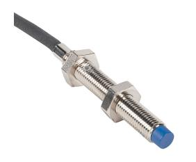
Micro Detectors inductive proximity sensor, tubular, 8mm diameter x 62mm body, nickel-plated brass housing, N.C. output, 4mm sensing distance, non-flush, 25 Hz (AC)/750 Hz (DC) switching frequency, IP67, pigtail.
