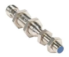
Micro Detectors inductive proximity sensor, tubular, 8mm diameter x 82mm body, nickel-plated brass housing, N.C. (VAC) or N.O./N.C. (VDC) output, 2mm sensing distance, flush, 25 Hz (AC)/900 Hz (DC) switching frequency, IP67, 1/2in - 20UNF thread.
