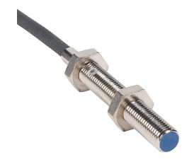
Micro Detectors inductive proximity sensor, tubular, 8mm diameter x 62mm body, nickel-plated brass housing, N.C. output, 2mm sensing distance, flush, 25 Hz (AC)/900 Hz (DC) switching frequency, IP67, pigtail.
