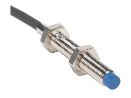
Micro Detectors inductive proximity sensor, tubular, 8mm diameter x 62mm body, nickel-plated brass housing, N.O. output, 4mm sensing distance, non-flush, 25 Hz (AC)/750 Hz (DC) switching frequency, IP67, pigtail.
