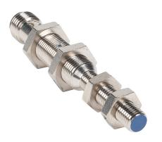
Micro Detectors inductive proximity sensor, tubular, 8mm diameter x 82mm body, nickel-plated brass housing, N.O. (VAC) or N.O./N.C. (VDC) output, 2mm sensing distance, flush, 25 Hz (AC)/900 Hz (DC) switching frequency, IP67, 1/2in - 20UNF thread.
