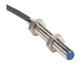
Micro Detectors inductive proximity sensor, tubular, 8mm diameter x 62mm body, nickel-plated brass housing, N.O. output, 2mm sensing distance, flush, 25 Hz (AC)/900 Hz (DC) switching frequency, IP67, pigtail.
