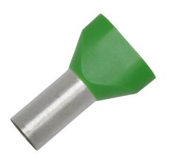
Z+F ferrule, 6 AWG, green, 2-wire, 16mm ferrule length. Package of 50.
