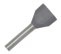
Z+F ferrule, 18 AWG, gray, 2-wire, follows DIN standard, 10mm ferrule length. Package of 500.
