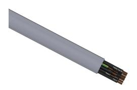
Southwire flexible control cable, unshielded, 25 conductors (includes ground), 20 AWG, bare copper, PVC/Nylon conductor insulation material, black with white numbers and green/yellow ground, TPE jacket, gray, cut to length.
