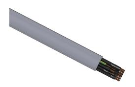
Southwire flexible control cable, unshielded, 25 conductors (includes ground), 20 AWG, bare copper, PVC/Nylon conductor insulation material, black with white numbers and green/yellow ground, TPE jacket, gray, cut to length.
