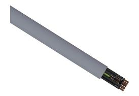
Southwire flexible control cable, unshielded, 18 conductors (includes ground), 20 AWG, bare copper, PVC/Nylon conductor insulation material, black with white numbers and green/yellow ground, TPE jacket, gray, cut to length.
