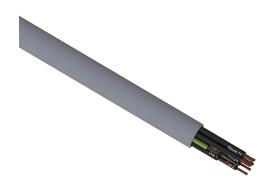
Southwire flexible control cable, unshielded, 12 conductors (includes ground), 20 AWG, bare copper, PVC/Nylon conductor insulation material, black with white numbers and green/yellow ground, TPE jacket, gray, cut to length.
