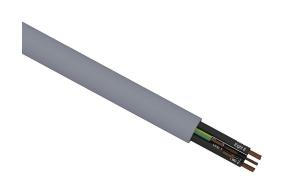
Southwire flexible control cable, unshielded, 9 conductors (includes ground), 20 AWG, bare copper, PVC/Nylon conductor insulation material, black with white numbers and green/yellow ground, TPE jacket, gray, cut to length.
