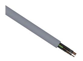
Southwire flexible control cable, unshielded, 7 conductors (includes ground), 20 AWG, bare copper, PVC/Nylon conductor insulation material, black with white numbers and green/yellow ground, TPE jacket, gray, cut to length.
