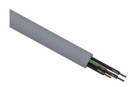
Southwire flexible control cable, unshielded, 5 conductors (includes ground), 20 AWG, bare copper, PVC/Nylon conductor insulation material, black with white numbers and green/yellow ground, TPE jacket, gray, cut to length.
