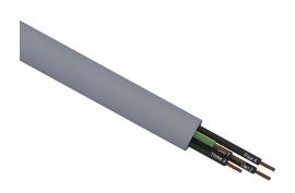
Southwire flexible control cable, unshielded, 5 conductors (includes ground), 20 AWG, bare copper, PVC/Nylon conductor insulation material, black with white numbers and green/yellow ground, TPE jacket, gray, cut to length.
